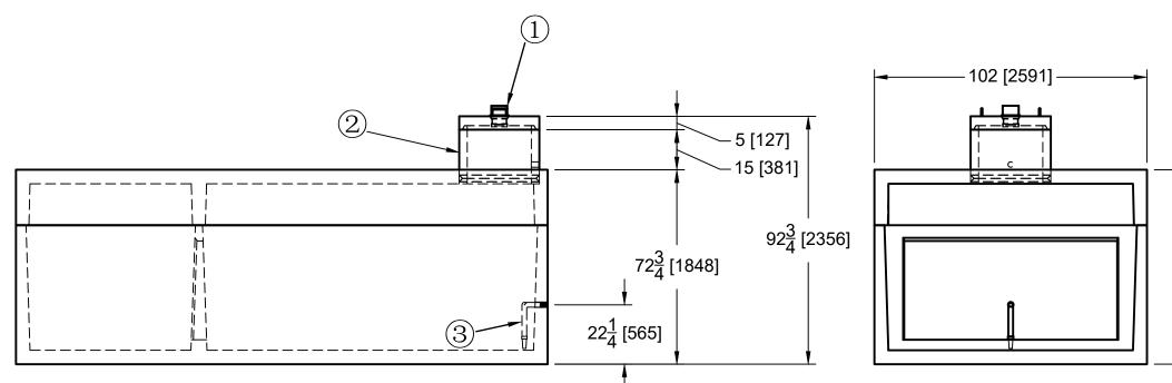
1: 6" PVC fill stack with removable cap 2:24"ID (30 OD) x 15" high riser with 2" conduit coupler + 5" high lid 3: 1-1/4" stainless steel coupler with footvalve pre-installed in tank
