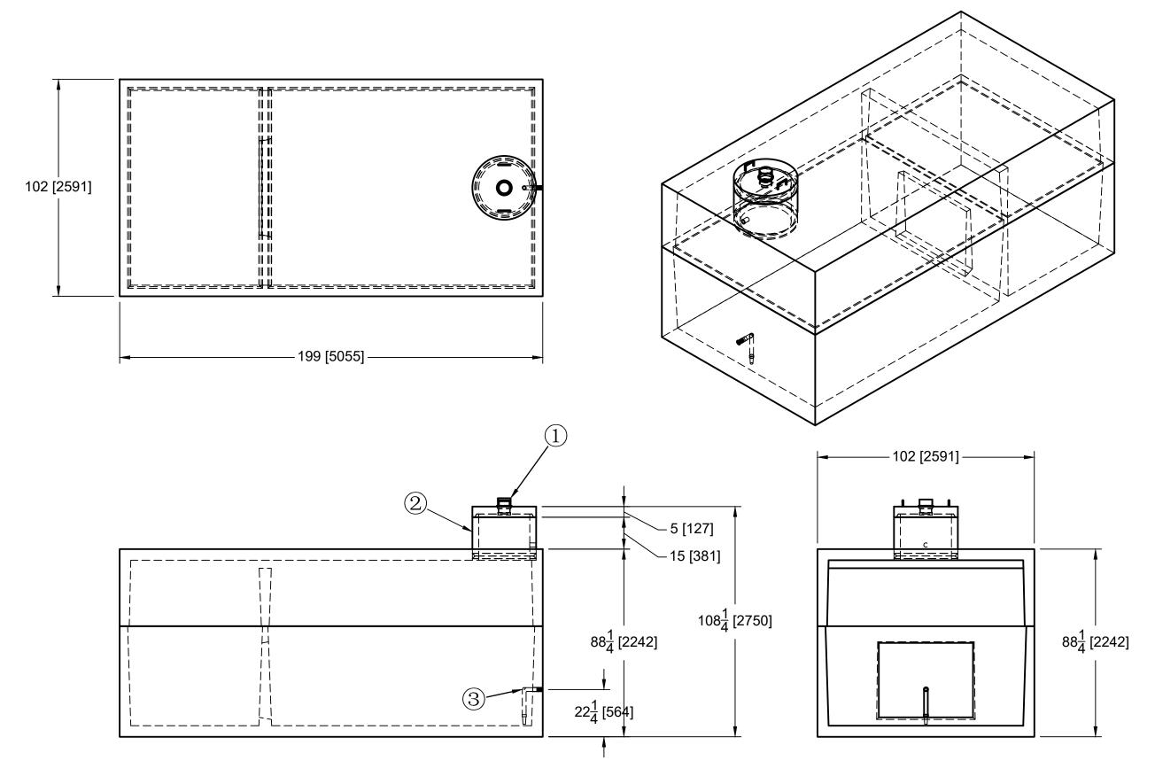
1: 6" PVC fill stack with removable cap 2:24"ID (30 OD) x 15" high riser with 2" conduit coupler + 5" high lid 3: 1-1/4" stainless steel coupler with footvalve pre-installed in tank
